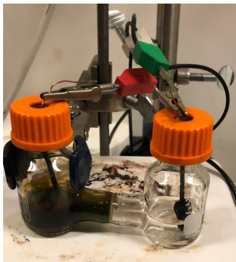
Figure C.1 Electrochemical acylation of indazole in an H-Cell performed with a 0.1 M solution of tetrabutylammonium hexafluorophosphate (TBAPF 6 ) containing 0.75 m mol of amine in acetonitrile in the cathode side and 0.75 m mol of ferrocene on anode side. Reticulate Vitreous Carbon electrodes were employed as cathode and anode.
