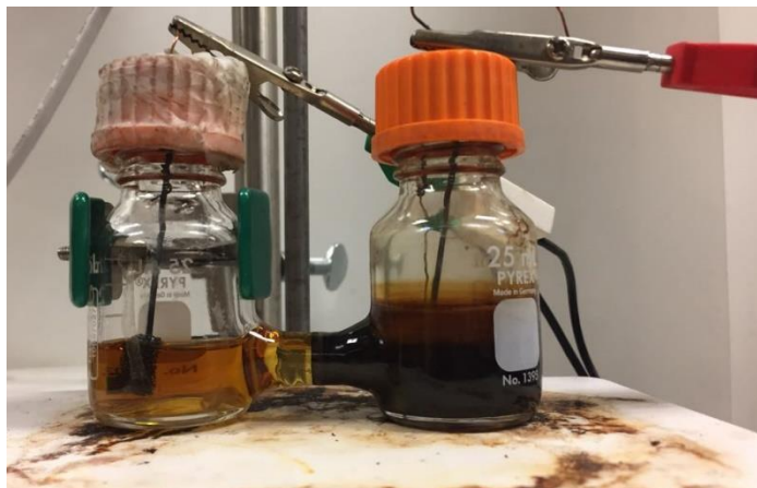
Figure B.2 Electrochemical acylation of indazole in an H-Cell performed with a 0.1 M solution of tetrabutylammonium hexafluorophosphate (TBAPF 6 ) containing 0.65 m mol of indazole in acetonitrile in the cathode side and 0.65 m mol of ferrocene on anode side. Reticulate Vitreous Carbon electrodes were employed as cathode and anode.
