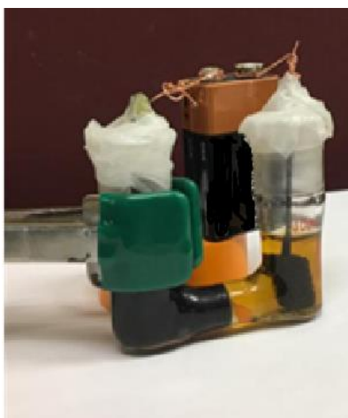
Figure C.2 Electrochemical acylation of indazole in an H-Cell performed with a 0.1 M solution of tetrabutylammonium hexafluorophosphate (TBAPF 6 ) containing 0.2 m mol of indazole in acetonitrile in the cathode side and 0.5 m mol of ferrocene on anode side. Benzoic anhydride (0.24 m mol) was added after 2 hrs. Reticulate Vitreous Carbon electrodes were employed as cathode and anode. Constant Current Electrolysis is carried out by connecting the electrodes to a commercially available battery.
